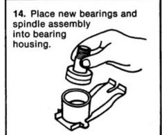
15. If inside of housing is clean and the bearings started straight, the bearing and spindle assembly should just slip in. If not, the use of a tube to push on the bearings outer race will ease installation.
