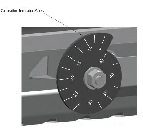
• Adjust material flow by rotating the cam wheel to either increase or decrease gate slide movement, see below.
