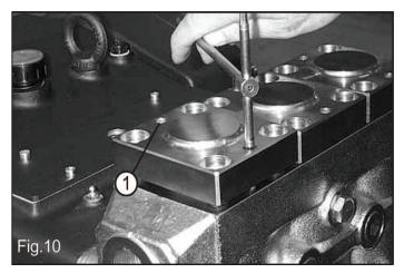
Tighten the two grub screws (1 Fig. 10) of each valve cover until the complete valve unit moves upward enough to allow easy extraction.
