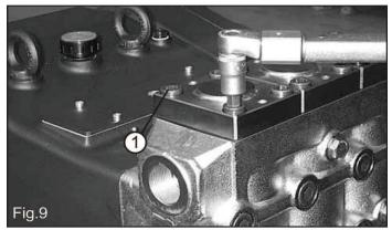
Loosen and remove the valve cover screws (1, Fig. 9).
