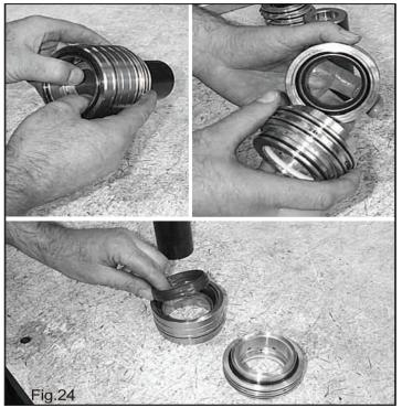
Separate the pumping unit components and check them for wear. Pressure packing replacement is carried out by hand without need for special tools (Fig. 24). A little bit of grease helps slide the packings into the packing support. Pressure Packings and o-rings should always be replaced at every disassembling of the pumping unit.
