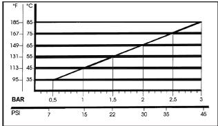
Naturally, if the application allows for feeding the pump with 45 psi (3 bar) even at low temperatures (for example: 115<sup>O</sup>F/45<sup>O</sup>C the life of the wet end of the pump will be even longer.
