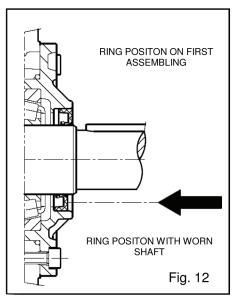
NOTE: Should the shaft show diameter wear in the seal position, it is possible to avoid grinding it by fitting the seal further as indicated in Fig. 12. Before installing the cover, (sight glass side) check the shim rings have been placed. To help the covers fit on the crankcase, you can use 3 screws M6 x 40, and then finish screwing them with the original bolts (M16 x 18).
