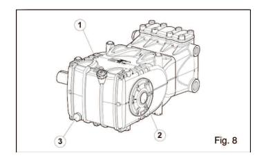
If necessary, add the missing oil through the oil plug (position 1, Fig. 8). Check oil level when the pump is at room temperature. When changing the oil (removing the plug position 3, Fig. 8), the pump should be at its working temperature.
