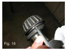
The new roller bearings can be mounted at room temperature with a press; it is necessary to hold them on the side surface of the ring nuts with suitable rings. The driving operation can be facilitated by heating the parts at a temperature between (250° - 300°F) making sure that the ring nuts are fitted in their seats.
