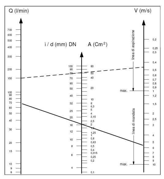
The diagram does not take into consideration the pipe and valve resistance, drop in pressure due to the pipe length the viscosity of the pumped fluid, its temperature, etc.
