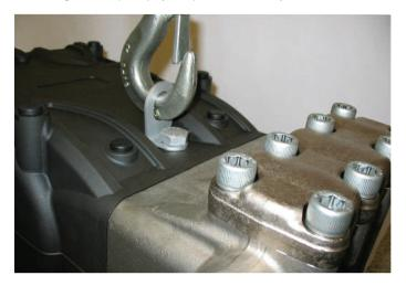
The eye bolt can be replaced with a plastic cap (see below), in order to protect the thread in the crankcase. The plastic cap is provided with the pump.
