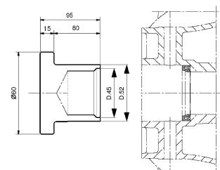
19.2 Piston guide oil seal assembling
