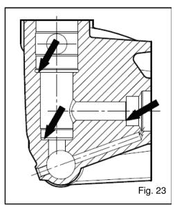
D) To reassemble the valves proceed the other way around and tighten the cover screws with a
