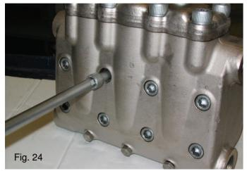
B) Remove the high pressure packings from the fluid end and the low pressure ones from their support by means of standard tools, taking great care not to damage the seats. See Fig. 25.
