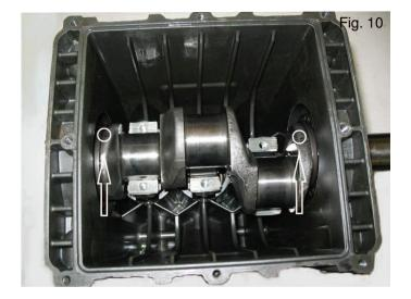
C) Disassemble the crankshaft oil seals and the piston guides using standard tools.
