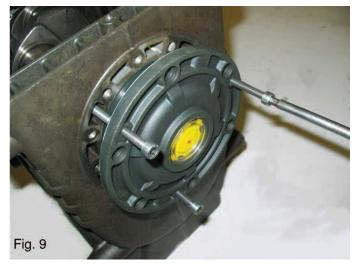
B) Push the piston guides and connecting rods forward so you can remove the pump crankshaft from the side. On the crankshaft, you will find marks (see Fig. 10) that must be turned towards the operator so the crankshaft can be easily extracted.
