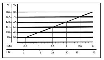
Naturally, if the application allows for feeding the pump with 45 psi (3 bar) even at low temperatures (for example:  $115^{\circ}F/45^{\circ}C$  the life of the wet end of the pump will be even longer.
