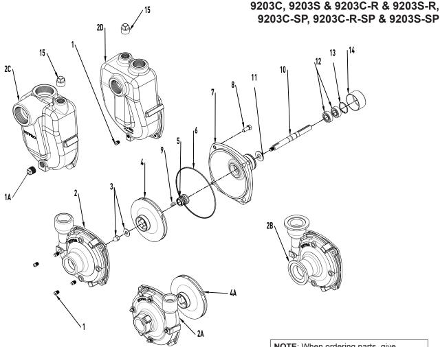
Silicon Carbide Seal Kit No. 3430-0589 consists of: (1) Ref. 5 Mechanical Seal (1) Ref. 6 O-Ring
