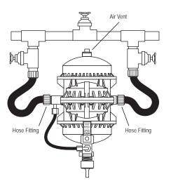
1. Make sure the water is turned off, and water pressure in the water motor is released - this is done by loosening the **Air Vent** (pressure relief valve) on the top of the water motor and turning off the water at both gate valves.
