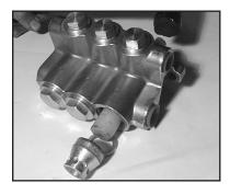
6. Remove the inlet valve retainer assembly (34A-39)
