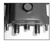
15. Before replacing pump manifold (29), first rotate crankshaft (18) until two outside plungers (24A) extend evenly forward. Next lubricate v-sleeves (50) in the rear v-sleeve housing (48) and slide housing over plungers. Lubricate ceramic plungers with a light film of oil. Carefully and evenly slide manifold over plungers and press manifold firmly against crankcase (1). Replace manifold stud bolts (45), washers (47) and nut (46) and tighten to 59 ft.-lbs.
