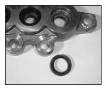
17. Lubricate the weep seal (50) and install into the intermediate casing (48).
