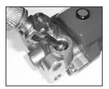
Use a slide hammer with a finger attachment to remove the valve seats (37).
