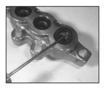
9. Remove and inspect the weep seal (50) and replace if necessary.
