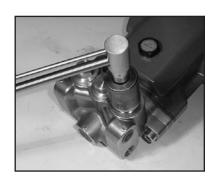
24. Replace the discharge plugs (43) and torque to 52 ft.-lbs (70 NM).
