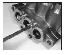
7. Using a 6mm allen wrench, remove the two inner hexagon screws (46).
