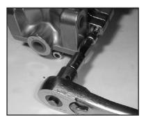
5. Using a 8mm allen wrench, remove the inner hexagon screws (45).
