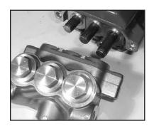
With a rubber mallet tap the back of the valve casing (29) and pull the valve casing (29) off the plungers (24A).
