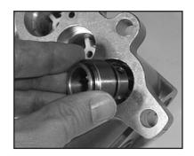
Install the seal case (39) with O-rings (40 and/or 40A) into the valve casing (29).
