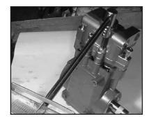
Place the valve casing (29) over the plungers. Secure the valve casing with the inner hexagon screws (45). Torque the screws to 33 ft.-lbs (45 NM).
