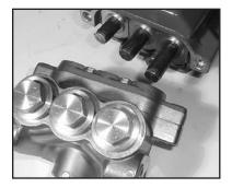
With a rubber mallet tap the back of the valve casing (29) and pull the valve casing (29) off the plungers (24A).
