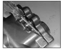
8. Separate the intermediate casing (48) from the valve casing (29)
