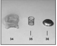
2. With a pair of needle nose pliers, remove the discharge valve cage (34), spring (35) and plate (36).
