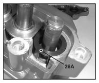
19. Replace the three spacer sleeves (26A) over the plunger with the flanged side toward the valve casing (29).
