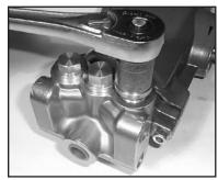
With a 22mm socket, remove the three discharge valve plugs (43) from the top of the manifold.
