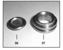
Inspect the valve seat (37) and valve plate (36) for signs of wear or cavitation and replace as necessary.
