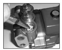
23. Install the three discharge valve assemblies with O-rings (34 - 38).
