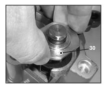
20. Install the pressure rings (30) over the plungers. Make sure that the O-ring (49) is in place.
