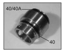
Remove the seal case (39) from the valve casing (29) and inspect both o-rings (40 and/or 40A) for wear.
