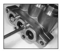
Secure the intermediate casing (48) to the valve casing (29) with the inner hexagon screws (46). Torque the screws to 107 in-lbs (12 NM).
