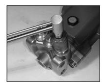
24. Replace the discharge plugs (43) and torque to 52 ft.-lbs (70 NM).
