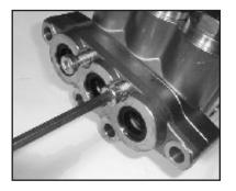
Using a 6mm allen wrench, remove the two inner hexagon screws (46).
