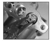
12. Using a needle nose pliers, remove the valve cage (34), spring (35) and valve plate (36) from the valve casing (29). Using a slide hammer with finger attachments, remove the valve seat (37) from the valve casing.
