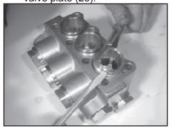
Using two screwdrivers, remove seal case (21)
