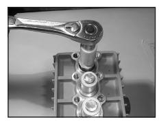
10) If the plunger pipe (16B) is worn, remove tension screw (16D) and remove along with plunger pipe (16B). Check and clean plunger surface (16A), check oil scraper (16H). Cover thread of tension screw (16D) with a thin film of Loctite and tighten carefully to 21 ft.-lbs. (28 Nm).
