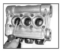
7) Remove the pressure rings (24) and v-sleeves (23) from the valve casing (26).
