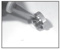
5. Apply one drop of Loctite 243 to valve plugs (#32) and tighten to 55 ft.-lbs. For pumps manufactured prior to 5/97 tighten plugs to 37 ft-lbs.
