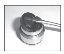
pumps, use a flat screw driver to pry the oil seals (#19) loose from the seal case (#20).
