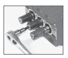
Clean the old sealant from the threads of the tension screw and the plunger base (#16A). Replace the copper washer (#16D). Place plunger pipes over plunger base and secure with tension screw to 199 in-lbs.
