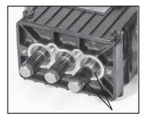
plunger bases and plunger pipes (#16B). A damaged surface will cause accelerated wear on the seals. Deposits of any kind must be carefully removed from the plunger surface. A damaged plunger must be replaced!
