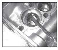
9. Remove the pressure rings (#24) and grooved seals (#23) from the valve casing (#26). Inspect parts for wear and replace if necessary. For P318, P324 & P330 only, the spacers (#23A) can now be removed.
