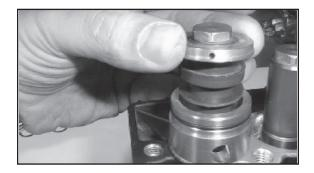
**15.** Place each seal case (#20) with o-rings (#21, 22) over the plungers (#16). Be certain the oil seal is centered with the seal case and tap firmly until the seal case is seated squarely on the crankcase (#1). Place pressure ring (#24) in seal case). **16.** With the grooved side pointed toward the valve casing, place the weep grooved seals (23A) over each plunger and into each seal case (#20).
