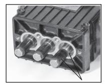
Check surfaces of the plunger bases and plunger pipes (#16B). A damaged surface will cause accelerated wear on the seals. Deposits of any kind must be carefully removed from the plunger surface. A damaged plunger must be replaced!
