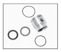
**11.** Inspect o-rings (#21 and 22) and replace as necessary.
