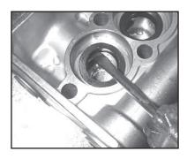
Remove the pressure rings (#24) and grooved seals (#23) from the valve casing (#26). Inspect parts for wear and replace if necessary.
