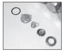
Remove each o-ring (#31). Inspect all parts for wear and replace as necessary. Reassemble valve assy's (32X) & place in valve casing (26)
