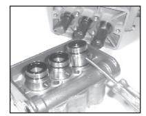
8. Remove weep return rings (#25) from the plungers (#16). Remove the seal case (#20) from either crankcases (#1) or manifold (#26) by using a screwdriver as shown above. NOTE: If there are deposits of any kind (i.e., lime deposits) in the valve casing, be certain the weep holes in the weep return ring (#25) and valve casing (#26) have not been plugged.
