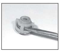
3. The valve assemblies can be separated by inserting a small screw driver between the valve seat (#27) and its valve spring retainer (#30).
