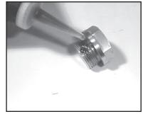
5. Apply one drop of Loctite 243 to valve plugs (32) and tighten to 59 ft.-lbs. For pumps manufactured prior to 5/97 tighten plugs to 37 ft-lbs.
