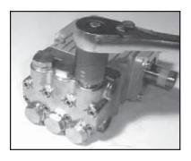
1. With a 22mm socket wrench, remove the (3) discharge valve plugs and (3) inlet valve plugs (32) Inspect the o-ring (33) for wear and replace if damaged.
