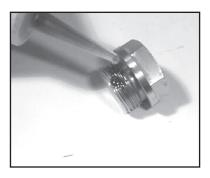
Remove the o-ring (31). Inspect all parts for wear and replace as necessary. For pumps manufactured prior to 5/97, tighten plugs (32) to 33 ft-lbs. otherwise, apply one drop of Loctite 243 to the valve plugs (32) and tighten to 55 ft.-lbs. (75 Nm).
