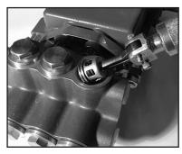
3. From the discharge port remove the spring retainer (#47) spring (#46) and the valve plate (#45). Using the valve puller (Available from Snap-On Tools) remove the valve seat (#44)
