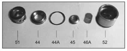
7. Pull the inlet valve assembly apart for inspection. Any resistance may be overcome by placing the valve housing (#52) in a brass jawed vise and carefully tapping the back of the valve plate (#45) with a screwdriver. Inspect the valve seats (#44), spring (#46A), o-ring (#44A) and o-ring (#53A for MP4120W/MP4124W) for wear and replace them as necessary.
