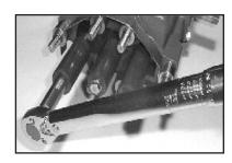
Torque the ceramic plunger bolt assembly to 300 inchpounds (34 Nm). If originally removed, reinstall the stud bolts (#49).
