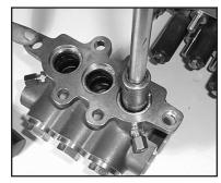
S. To remove the inlet valve assembly, insert a 13mm socket with extension through the rear of the inlet manifold (#43) port and tap it firmly with a hammer. This will force the tension spring (#46A), valve housing (#52) and the remainder of the inlet valve assembly out through the front of the inlet port.
