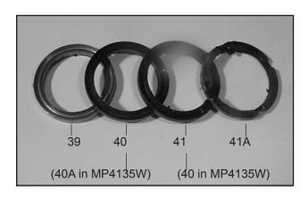
Reinstall the pressure ring (#39), v-sleeve (#40 / #40A fpr MP4135W), support ring (#41 / #40 for MP4135W) and intermediate ring (#41A) into each plunger bore. Re-install the tension spring (#42). For MP4120W/MP4124W only replace the spacer ring (#52A).
