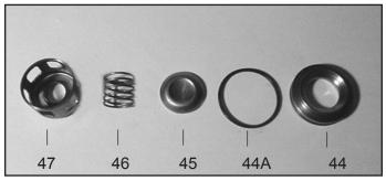
Inspect all parts, especially the seating surface of the valve plate (#45), and replace as necessary.
