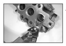
15. Replace the rear support ring (#35A for MP4120W/MP4124W and #41 for MP4130W/MP4135W). Replace the rear v-sleeve (#35B for MP4120W/MP4124W and #40 for MP4130W/MP4135W) and rear pressure ring (#35C for MP4120W/MP4124W and #39 for MP4130W/MP4135W) making sure that the grooved side is facing the discharge end of the manifold (#43). For MP4120W/MP4124W, replace the rear o-ring (#35D) into the back of the manifold (#43). Replace the snap ring (#36).
