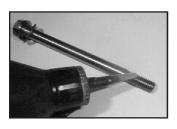
13. Clean the bolt threads (#29C), apply locktite, and remount.
