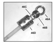
4) Loosen valve seats (46A) and valve spring (46C) from spacer pipe (46D) by lightly hitting the valve plate (46B) with a plastic stick. LP600/LP600-4000 pumps have an additional valve spring guide (46E). Check sealing surface and replace worn parts. Reassemble with new O-rings (44A) if possible and oil them before installing.
