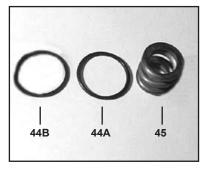
2) Remove the support ring (44B), O-ring (44A) and tension spring (45).
