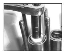
11. Tighten the tension screws (29C) to 310 in.lbs. (35NM). The plunger pipe (29B) should not be strained by over tightening of the tension screw (29C) or through damage to the front surface of the plunger; otherwise, it will probably break.
