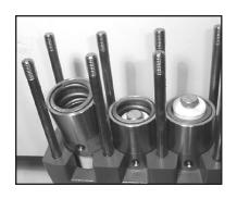
6. Pull seal sleeves (35) out of guides in crankcase (1).
