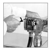
To remove the nutator disc, loosen the two screws holding the disc in the meter housing and lift the disc and O-ring from the main meter housing. (Figure 9)
