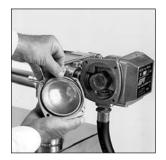
4. Hold the coverplate in position and replace the four screws by alternately tightening screws until the coverplate is firm against the meter housing.
