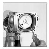
NOTE: It may be necessary to place a screwdriver under the edge of the nutator and gently pry free.
