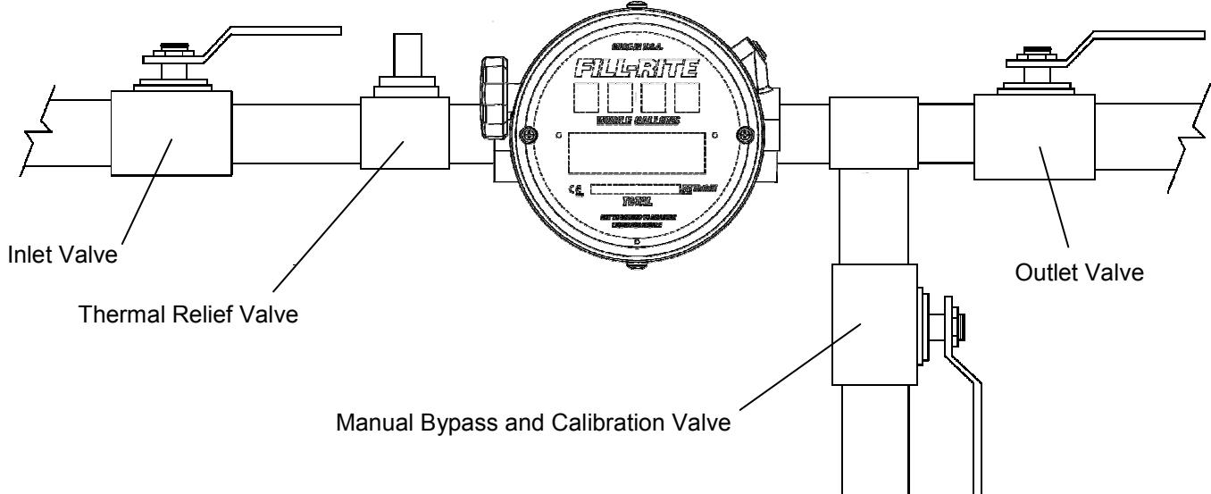
Positive displacement (PD) meters are designed to operate full of liquid. The meter should be installed in a location, where it remains **full of liquid** at all times. It may be installed in vertical lines, provide that liquid flows up.
