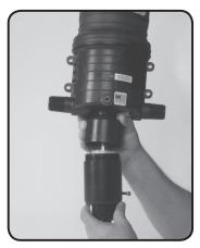
Step 1. Unscrew LOWER END ASSEMBLY from body.
