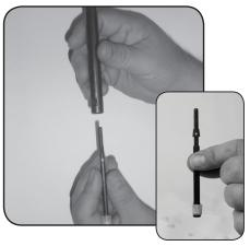
Step 5a. For 0.3%. Replace LOWER SHAFT assembly into upper shaft.
