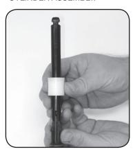
Step 4. For 2.5% & 5% Replace #44 DOSAGE PISTON flared-end up and #14 O-ring. 0.3% only: Replace #51 SHAFT ASSEMBLY. See Step 5a.
