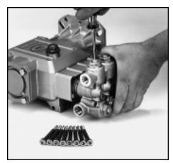
Separation of Manifold Head from Crankcase
