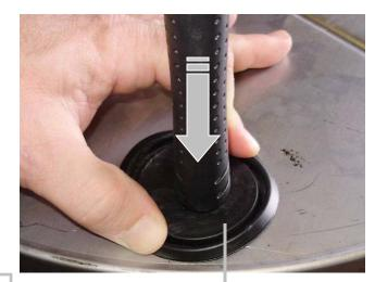
To insert 5871B8 cap plugs into bottom holes, pinch cap plug into place using index finger and thumb. With edges of plug resting against edges of hole, firmly push down on plug with end of hammer or other blunt object until plug snaps into place.
