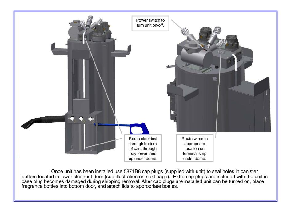
To attach hose, thread into metal hole counter clockwise.
