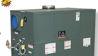
Models WH989/H989 are rated at 990,000 btu input. Output is 842,000 btu for water heaters and 832,000 btu for boilers. Dimensions are 57" wide x 33" deep x 41" high. Shipping weight, 900 lbs.
