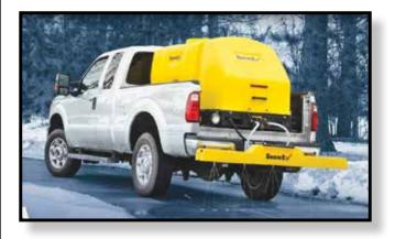
VSS1000 is designed for utility vehicles or compact pickups. 100 Gallon capacity. Standard with hose reel, spray wand and 50' of hose in addition to 3 nozzle boom for confined areas and stairways. Floor dimensions are 45" L x 32" W x 50" H. Spraying width is 6'. Capacity is 20 gallons per acre at 10 mph. Pump on/off switch with molded plug.
