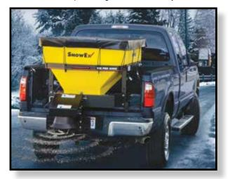
SP3000 1/2 cubic yard (1080 lbs.) and SP6000 1 cubic yard (2160 lbs.) models will handle bagged rock salt and bulk salt as is. Can also apply bagged ice melters, calcium flake and calcium chloride pellets with TRK3000 material control tube. Floor bed dimensions are 58" L X 34" W (SP3000) and 44" W (SP6000). Overall length is 77" L and 48". Spreading width up to 40'.
