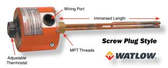
**Commercial Grade, Screw Plug Heaters** are intended for direct immersion to heat a variety of fluids to specific temperatures. The heater element is designed to be installed into a female threaded port in an existing tank or vessel.
