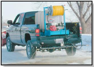
DU 1A202 Skid Mount Spray Package with 200 Gallon Tank and PB80R Boom
