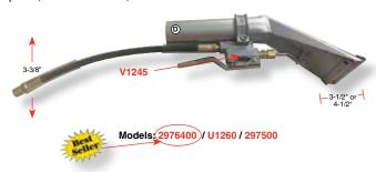
**Features:** All Stainless Steel construction • Designed for 1-1/4" or 1-1/2" vacuum hose as noted • Valves are rated to 400 psi. 2976400 & U1260 have 3-1/2" wide head. 297500 has 4-1/2" head. Length is 10". All wands are rated to 200° F.
