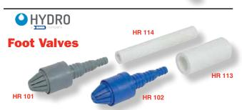
HYDRO FOOT VALVES allow one-way flow of chemical concentrations. Prevents solutions from "back-flowing" into supply tubing. Constructed of corrosion-resistant plastic and rubber materials for longer life. Polypropylene bodies with EPDM or Viton® diaphragms. (EPDM is recommended for Butyl base chemicals found in some tire cleaner products).
